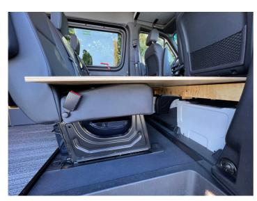
Platform folds out and rests on a custom mount that sits on the front seat rails. Push your front seats back and it's very secure.
