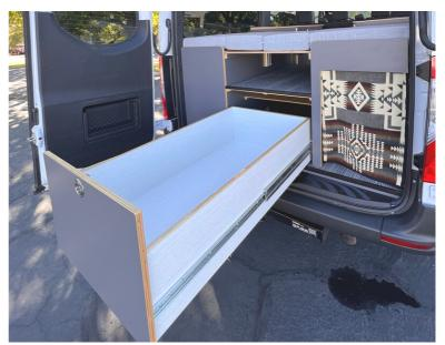
4ft Rear Pullout Gear Drawer with a hidden table pocket. 400lb capability. Southco Lock. Includes 2 keys.
